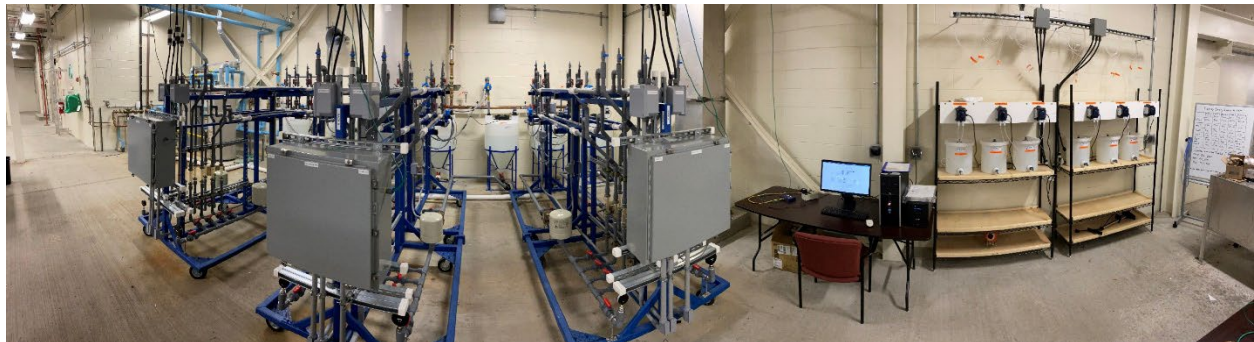
Lead Pipe Rig Corrosion Control Treatment Experiment
